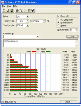
2. In terms of real world data transfer performance, a 7.98GB file is transferred between the HE720 to a desktop computer via USB 3.0 interface to the read/write speed. Based on the results of ATTO Disk Benchmark, the write speed can reach 107 MB/s, while the read speed can reach 109 MB/s.
